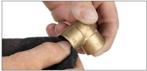
While being heated a layer of oxide will form on the copper surface, impairing the soldering. A third substance is needed to remove oxide formation.
